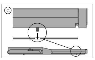
Then slot the front studs of the shelf into the slots provided in the front section of the runners. You must jiggle the shelf in order to slot the studs into the holes. Start by inserting the left stud. The right one will then slot naturally into the oblong hole.
