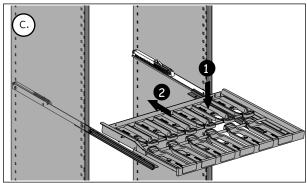
Position your shelf along the left and right runners and start by securing the rear section of the shelf.
