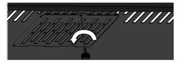
Unscrew the button of the charcoal filter hatch, under the control panel.
