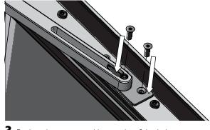
**2** Move forward the hinge attachment by one notch on the right.
