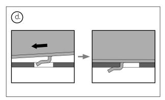
Slide the shelf until the rear hooks of the shelf are locked into the slots provided in the runners.
