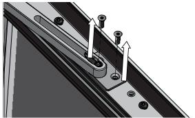
Remove the screws fastening the hinge to the door using a T25 screwdriver.
